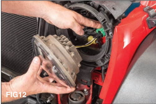
Carefully stow the wiring into the headlight bucket area. Be careful not to pinch any wires. (FIG 12)
