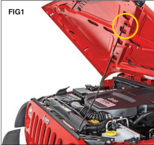
Put on safety glasses. Open the hood of your Jeep®. Put the prop rod into the correct slot to hold hood open (FIG 1).
