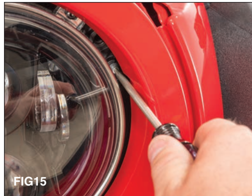
Always check the aim of your headlights before driving and adjust as needed using a T15 torx on the adjusting screws. (FIG15)
