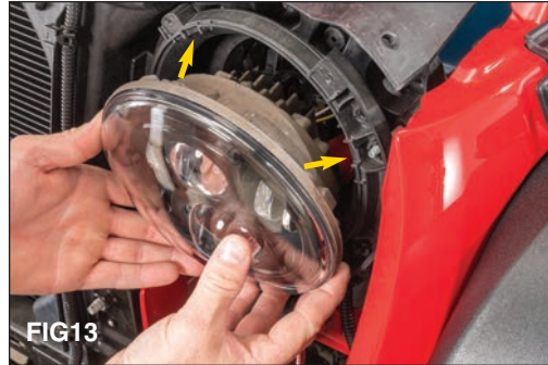
Align the three tabs on the back of the headlight with notches in the headlight bucket. (FIG 13)
