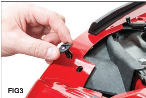
Depending on your model year, pry up or unscrew the plastic fasteners (6 total) using a small screw driver. Early vehicles may feature phillips head screws, but most vehicles have a pry-up rivet as shown (FIG 2). First remove the center, then remove the body of each plastic retainer (FIG 3). Set rivets & screws aside in a safe place for re-installing the grille.
