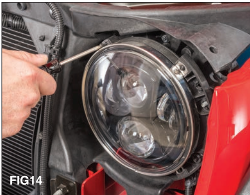
Reinstall headlight trim ring using factory T15 torx screws. (FIG 14) Repeat all above steps for the passenger side headlight. Reinstall the Grill, turn signals, etc. in the reverse order of the disassembly.
