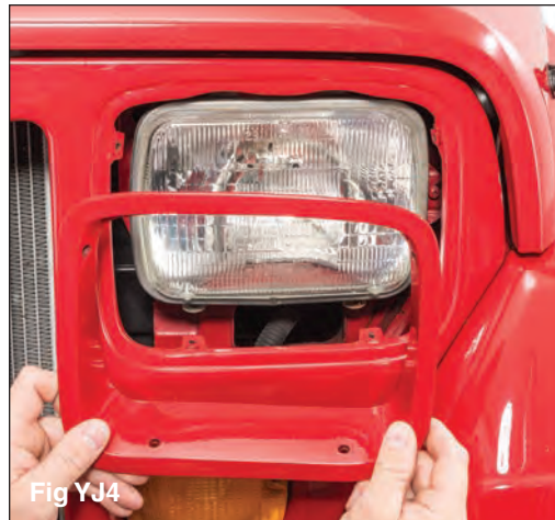
With the headlight bezel removed, the inner headlight retaining ring will be revealed. (see next page)
