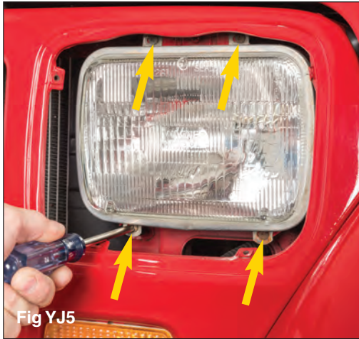
Remove the headlight retaining ring by removing the 4 Phillips Head screws as shown in Fig YJ5. Safely set aside the screws for re-installation.
