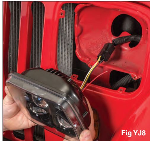
Plug in the new LED headlight. (FIG YJ8) Position the headlamp to sit flush in the headlight bucket.
