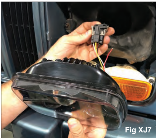
Plug in the new LED headlight. (FIG XJ7) Position the headlamp to sit flush in the headlight bucket.
