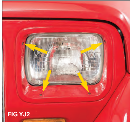
Remove the headlight bezel by first removing the four screws using a Phillips Head screwdriver shown in FIGs YJ2 and YJ3.
