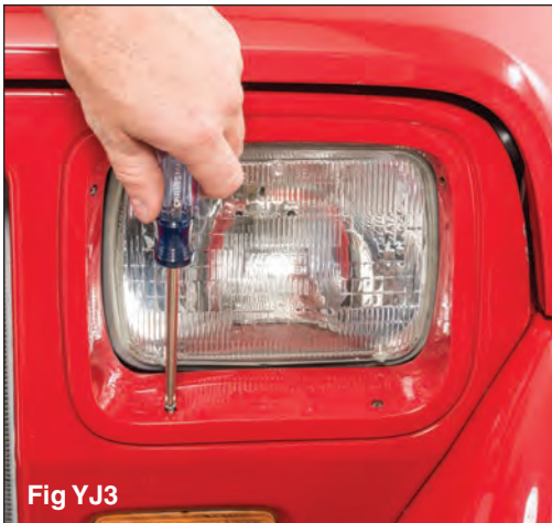
Remove the headlight bezel as shown in FIG YJ4 and set it down carefully with the factory Phillips screws for reinstallation.
