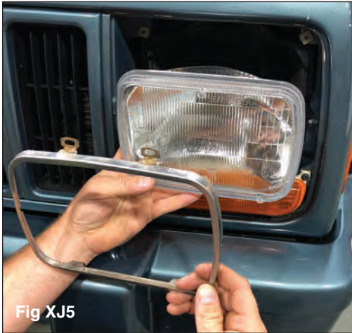
Remove the headlight retaining ring, then unplug and remove the stock headlight as shown. (FIGs XJ5 & XJ6)
