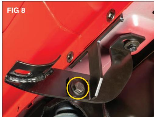
Next align the mounting slots between the two brackets and loosely install a 10mm bolt (A) with washers (G) on both sides and secure with a 10mm nylock nut (E) using a 16mm hex wrench and a 17mm socket. (FIG 8)
