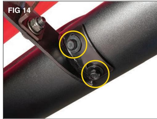
Loosely install the 8mm bolt with captive washer (D) using a 13mm socket. (FIG 14)
