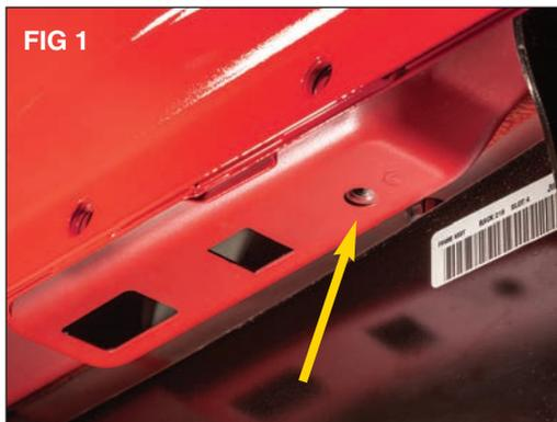
Put on safety glasses. Starting at the front of vehicle locate the vertical threaded hole behind the pinch weld. (FIG 1)
