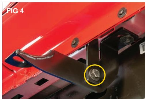
Next align the mounting slots between the two brackets and loosely install a 10mm bolt (A) with washers (G) on both sides and secure with a 10mm nylock nut (E) using a 16mm hex wrench and a 17mm socket. (FIG 4)
