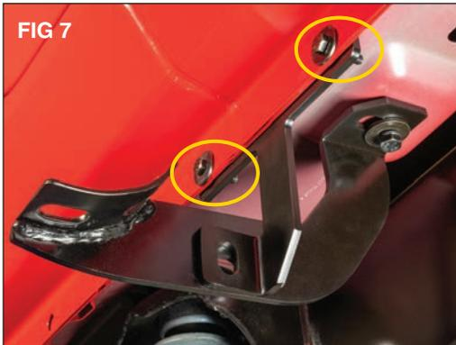
Locate and loosely install the center support bracket using 6mm hex head bolts (B) through the pinch weld with washers (I) on both sides and secure with a 6mm nylock nut (F) using a 10mm hex wrench and a 10mm socket. (FIG 7)
