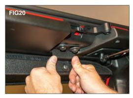
Now push the light brackets forward until they rest against the plastic trim. (FIG 20) You may now tighten the factory T-40 screws. Some adjustment may be necessary to re-align the brackets to your top latches.
