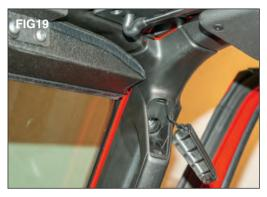
Re-install the grab handle taking care not to pinch any wires. (FIG 19) Also, Re-install the speaker cover.
