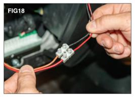
Using a small flat blade screwdriver connect the light bars harness to the power tap harness. (FIG 18) You may now reinstall the glove box in the reverse order.
