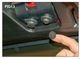
Unlatch and open the soft top or remove hard top front panels. Remove the felt padding on top of the brackets hardware. (FIG 13)
