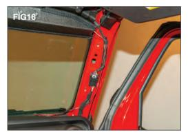
to the brackets using the supplied T-40 torx bolts and washers. Now, route the wiring harness as shown down the A-pillar along side of the factory wiring. (FIG 16)
