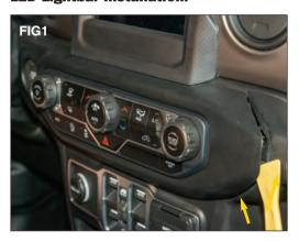
Put on safety glasses. Using a trim clip removal tool gently remove the center dash control center (FIG 1)
