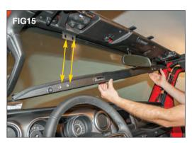
Tilt the light bar into place, careful not to knock off the smaller end gaskets. (FIG 15) Loosely attach the light bar
