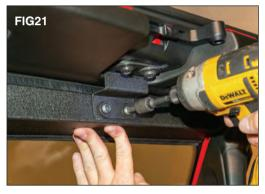
Finally, push up on the light bar and tighten the T-40 screws from bracket to light bar. (FIG 21)
