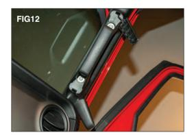
Remove the two bolts using a 10mm socket. (FIG 12) Remove handle and set it aside.
