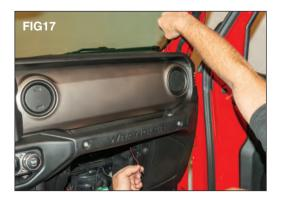
Fish the harness down through the dash to behind the glove box. (FIG 17)
