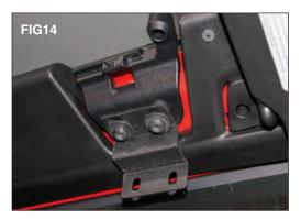
Remove the hardware using a T-40 Torx socket and loosely install the supplied brackets as shown. (FIG 14)
