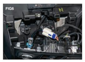
Connect the white connector to the original plug you just disconnected in FIG5. Connect the gray connector back into the 12v socket. (FIG 6)
