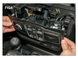
Gently pry out the window control panel from the top and work your way down. (FIG 4)
