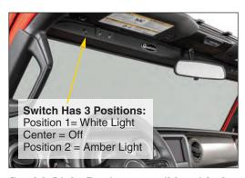
Stealth Light Bar is compatible with the standard rear view mirror as well as the auto-dimming version (above right).
