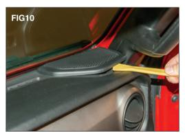
Using a trim tool gently pry up on the dash speaker cover and remove it. (FIG 10)
