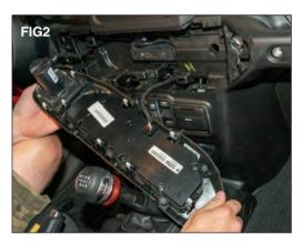
Disconnect any wiring harnesses and set control panel aside. (FIG 2)
