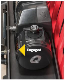
There are two positions of the clutch handle. The Clutch is either "engaged" or "free spooling". Clutch allows operator
