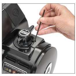
Rotate Clutch Handle to the "FREE SPOOL" position to reveal the set screw that holds the handle in place. Using a 2.5 MM Allen wrench, back out the set screw until the Clutch Handle lifts off but do not remove the handle at this time.
