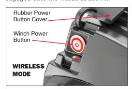
In the event of an emergency, the winch Power Button can be pressed to stop winch rotation. It will stay depressed and the drum light will blink indicating that the winch is in safe mode and will not rotate. Press the Power Button again to restart, wired operations (it will remain out).
