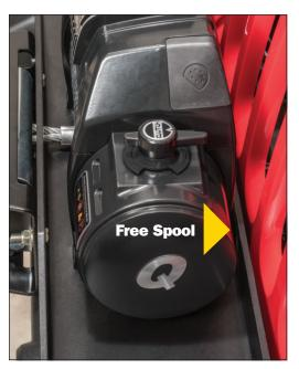
to manually engage or disengage the spooling drum from the gearset using the clutch lever.
