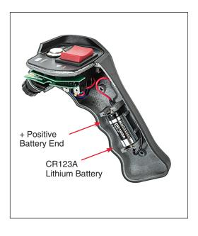
Carefully remove the old CR123A or CR123 Lithium battery and replace with new. Gently align and position the winch controller halves together and fasten the three Phillips head screws. Do not over tighten! Test the winch "OUT" and "IN" functions on the remote to ensure that the remote is functioning properly.
