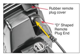
the remote handle to ensure a proper connection. Next, loosen the Rubber Plug Cover on the right hand side of the winch. Plug the "D" shaped end of the Remote Cord into the corresponding receptacle on the right hand side of the winch. Be sure that the plug is fully engaged onto the winch as shown.
