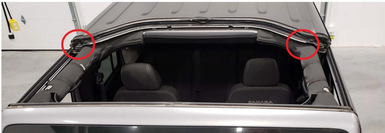
2. Place the panel on the top of the vehicle. Do not remove the protective film from the clear roof panel until the installation is complete. Only peel back the protective film as far as necessary to install the clear roof panel.
