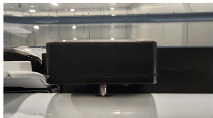
8. The rubber damper should be placed between the handle and the roll bar to prevent scratching your factory paint. It's important to note that a slight gap between the roll bar and the screw plate is entirely normal, do **not** over-tightening the components.
