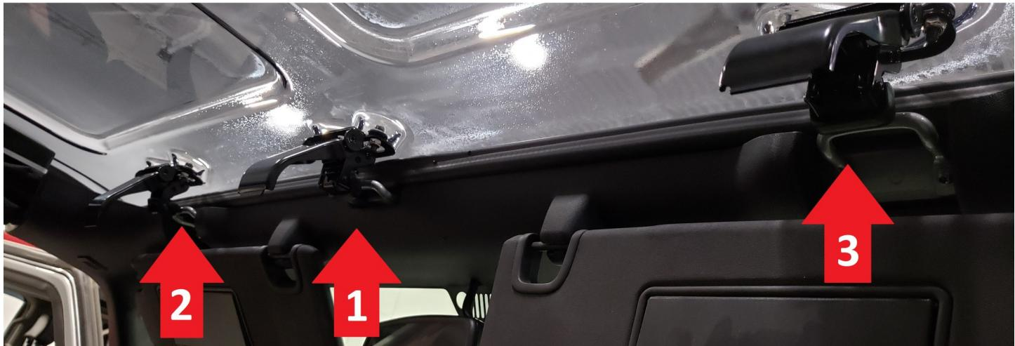
6. Starting at the rear of the vehicle, slowly tighten the hand bolts in the order shown below. Do not over tighten.
