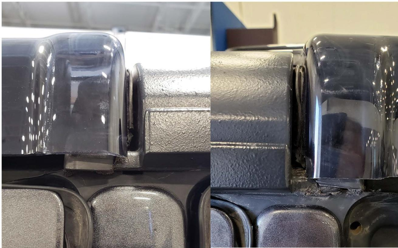
4. Insert the six stainless steel hand bolts through the roll bar and loosely thread them into the six adapter plates. The two stainless steel hand bolts without the rubber vibration dampers go in the rear holes shown below.
