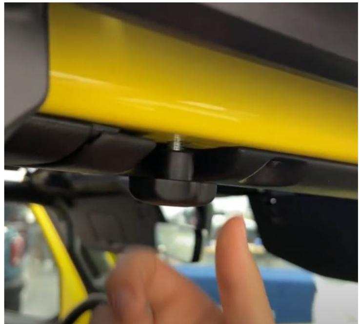
4. Tighten the M8 knobs leaving a small gap between the SkyLite hardware and the roll bar on the vehicle. Do not overtighten.
