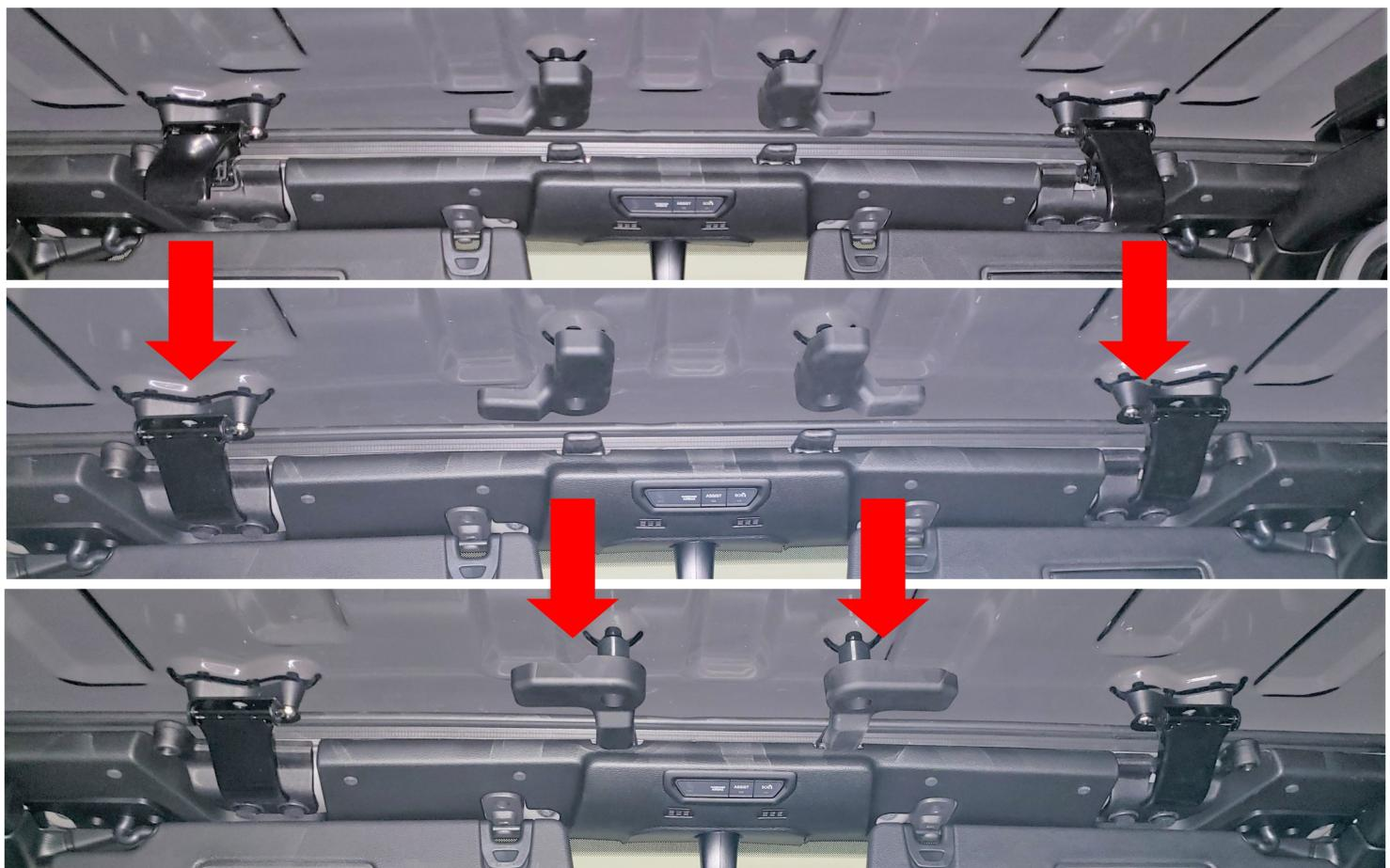
6. Close the rear two L-shaped clamps. (picture pointing to the rear clamps)
