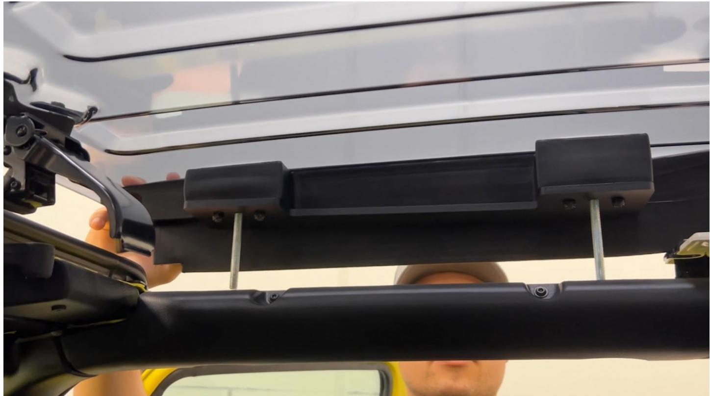
**Caution:** Leave the RED bolt covers on while installing the SkyLite to avoid scratching paint while installing the SkyLite lid.
