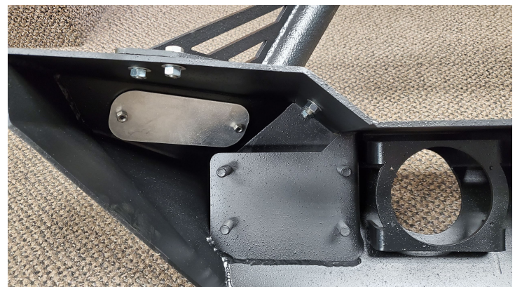
Detail 15: Accent plate & bull bar installed
