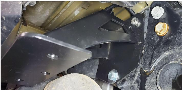
Detail A2: Install driver side mount bracket
