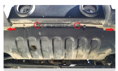
Detail 1: Remove lower push clips
