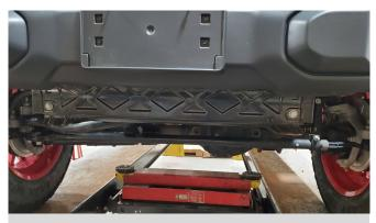
Detail 3: Remove bolts on brace
