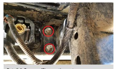
Detail 4: Remove (8) mounting nuts
