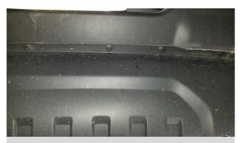
Detail 1: Remove lower push clips
