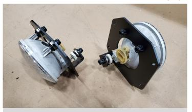
Detail 12: Install fog lights into adapter brackets
