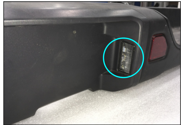
16. Remove the license plate lights. Disconnect license plate lights connector.
