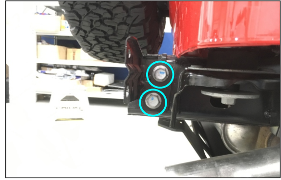
8. Unscrew bumper bracket's 2 fitting bolts on the right side of the vehicle.
