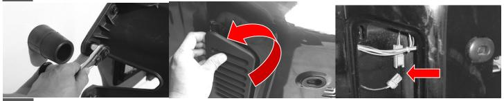
Press down on the plastic clip and then unplug the 3rd brake light wiring harness and remove along with the pass through grommet. You can find many creative ways to re-purpose this light if you search online if you like.
