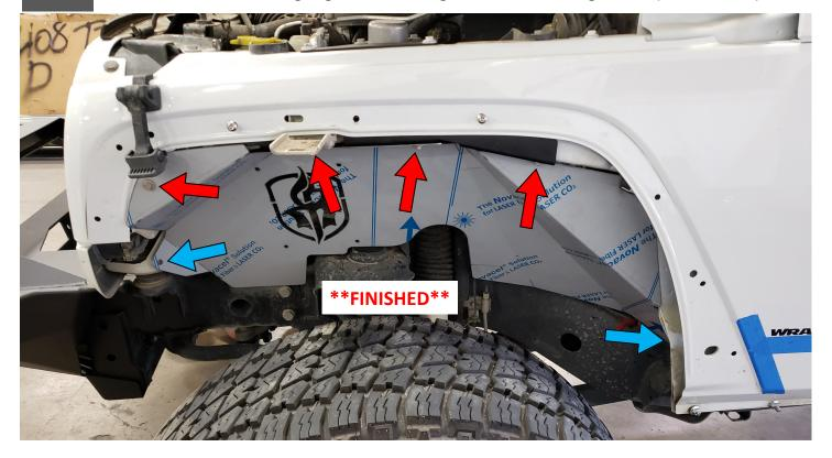
\*\*Remove protective film after fenders are installed.\*\*
