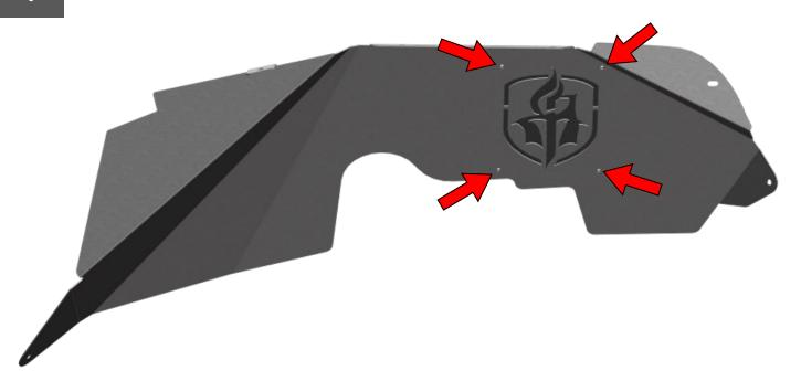
Install RA inner fender liner using four OEM bolts previously removed. (RED Arrows)
