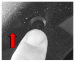
Remove six (6) 10mm Bolts inside fender well and all plastic fasteners. Keep all bolts for future use.
