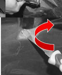
\*\*ALWAYS test fit/install fender liner prior to custom painting to ensure proper fit.\*\*
