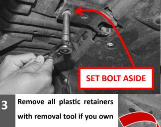
Remove all plastic retainers with removal tool if you own one, or carefully with a pair of dykes or a thin pry bar.
