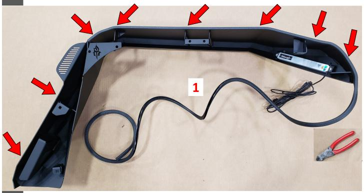
Install FENDER FLARE by inserting 2 - 5/16" CARRIAGE BOLTS into bottom rear holes first.
