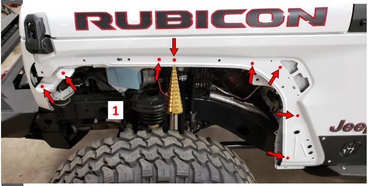
Install 8" ACCENT LIGHT into FENDER FLARES using 2 - #10-24 BOLTS and FLANGE NUTS.
