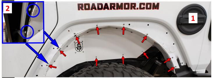
Install two NUT COVER PLATES shown in location above. (Between inner seam and 5/16" nuts.)
