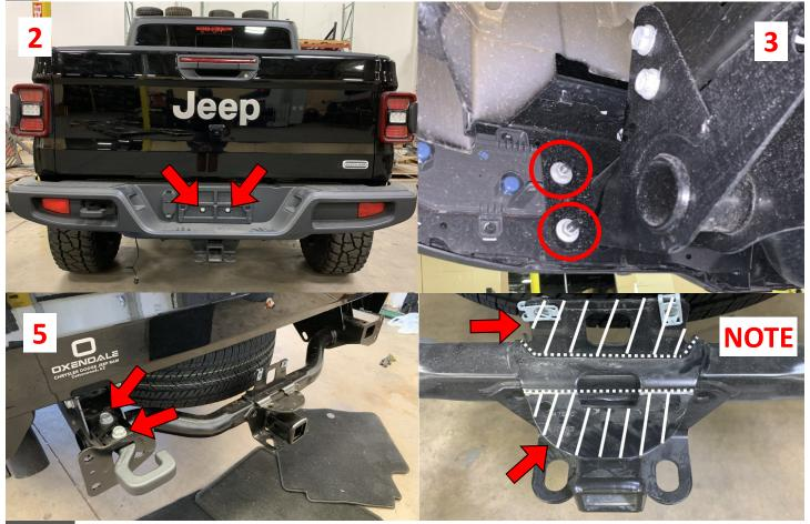
If equipped, disassemble rear bumper, carefully remove all sensors and harnesses. \*\*Note sensor location\*\*
