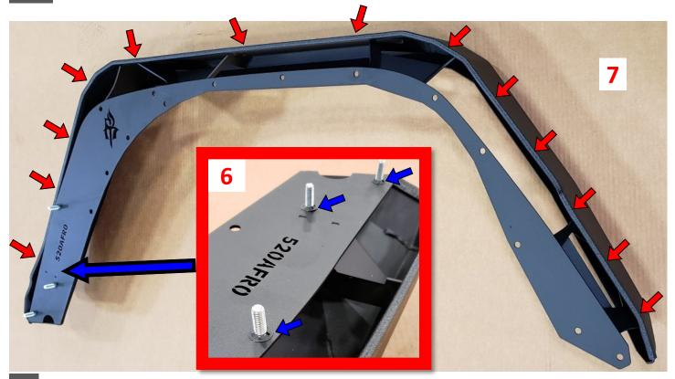
If installing <u>without</u> inner fender liners place fender onto bed seam by aligning 5/16" carriage bolts. Loosely install pinch seam bolts using 7 - 5/16" button-head bolts; (BLUE Arrows)
