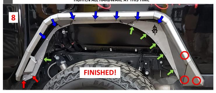
If installing RA Fenders <u>with</u> Inner Liners (520LFR0Z), refer to steps below. Assemble fender liners using 9 - 5/16" button-head bolts and flange nuts; (GREEN) NOTE: TRIM CIRCLED BOLT FLUSH WITH NUT FOR CLEARANCE ( followed by 11 - 5/16" U-nuts as shown below: (RED) Install RA - Logo backing plate using #10 hardware. (ORANGE) Install 2 - 5/16" U-nuts onto rear pinch seam as shown below.
