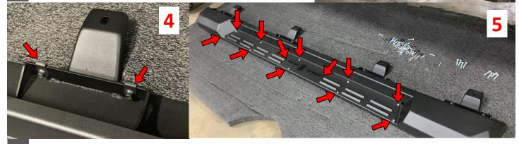
Install steps by aligning steps to pinch seam holes; supporting step with block of wood on floor jack. Install all 5/16" bolts & Sml. Washer through pinch seam & U-Nut clips into RA-Steps as shown. (RED) Install all M8 x 30mm bolts & Lrg Washer through RA-Steps landing pads and bottom of Jeep. (BLUE)
