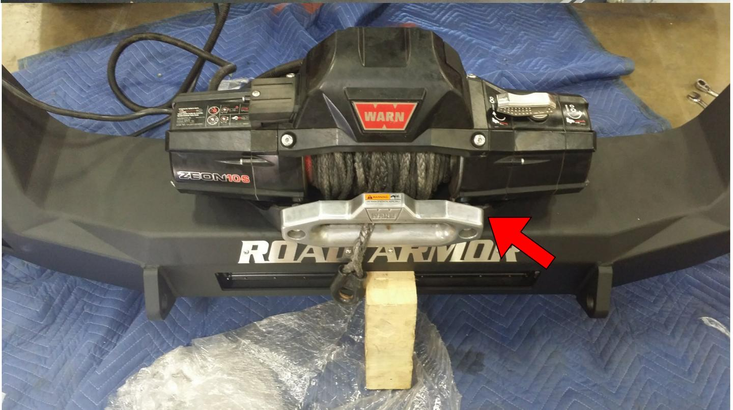
**14** Install bumper onto frame-horn lining up ALL holes and each 1/2" bolt tabs through frame. Then place the factory inner and outer stiffeners, which you were instructed to set aside in Step 5, followed by a washer (**Large**), lock-washer and nut on the backside finger tight. Repeat for Dvr.
