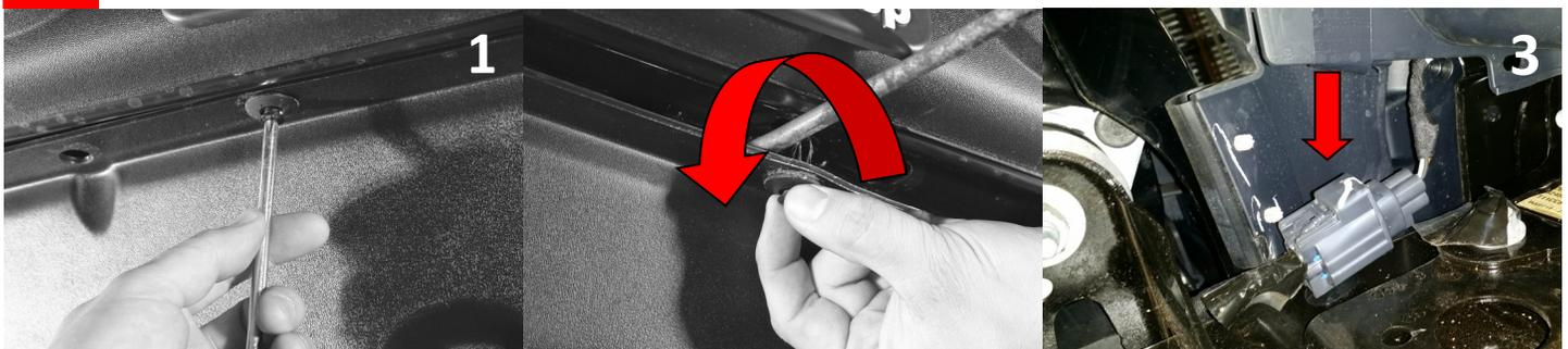
**2** Unscrew two (2) bolts on the bottom side of the front splash shield and remove.
