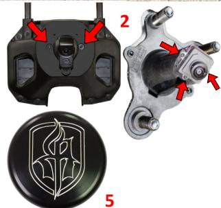
Once all weight has been added to carrier, check spindle nut torque, apply light amount of grease to inside of housing and threads to prevent rusting or moisture build-up. \*\*Secure RA-LOGO-CAP\*\*
