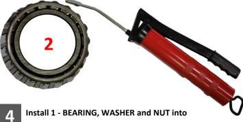
SPINDLE BRACKET as shown below . Use 36mm socket to secure the SPINDLE NUT.
