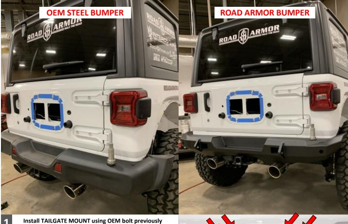
Install TAILGATE MOUNT using OEM bolt previously removed as shown:
