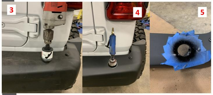
JL Rear Bumper will require the removal of sheet metal section below, mark, cut/remove, and paint edges as shown:
