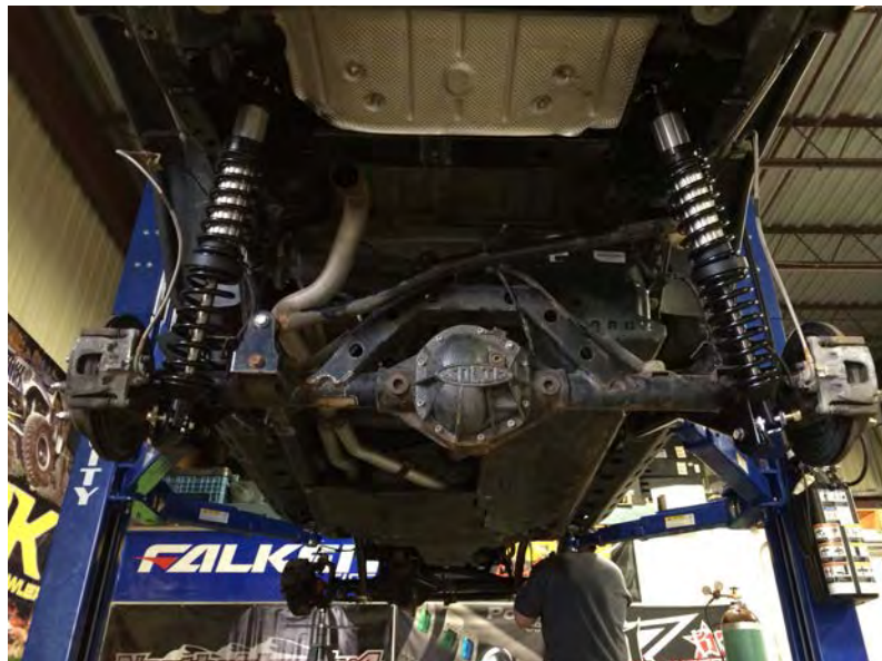
Emulsion Coil Over Install
