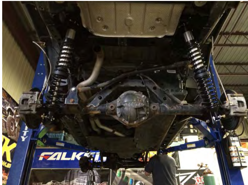
Emulsion Coil Over Install
