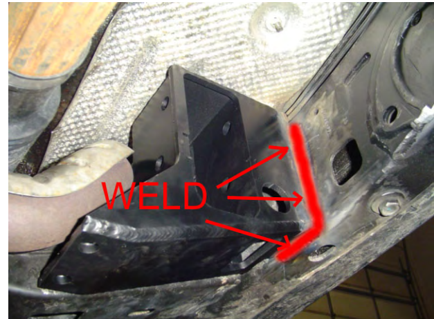
D.S. Bracket Welded in Place
