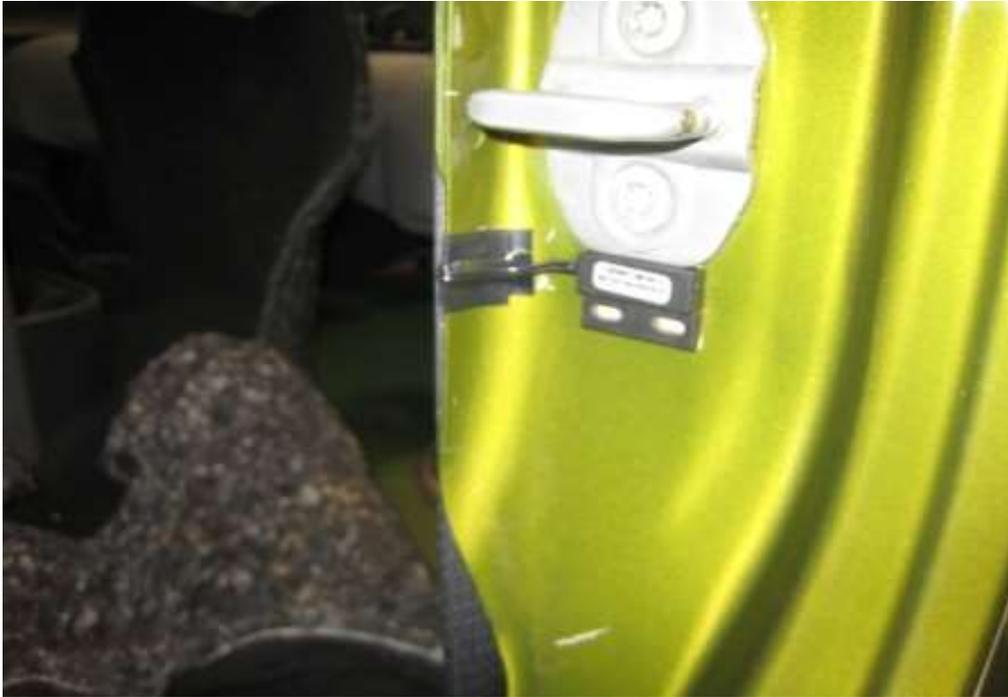
5. Divide the harness between the driver and passenger side. Mount the sensors on the driver and passenger side just underneath the door latch on the inside door frames using the sticky pads provided. Route the wires around the body seam by placing a small piece of electrical tape on the body seam. Wrap the wire over the top of the tape towards the inside of the cab then secure the wire with another piece of electrical tape. (shown above)
