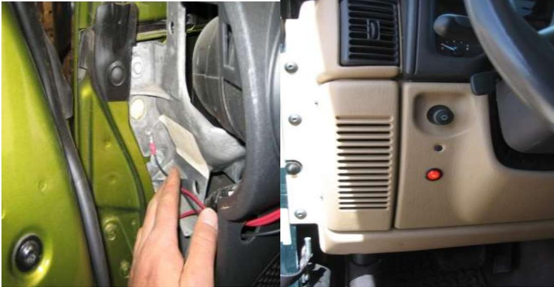
10. Route the POS+ and NEG- wires through the firewall on the driver side. ***Make sure not to interfere with any of the pedal linkage under the dash.***
