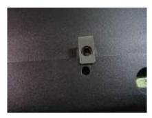
2. Place the skid plate with bolt holes against the bumper and so the skid plate is hanging down. Put washers on the bolts and insert bolts into their respective holes. Tighten bolts
