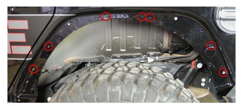
Install the rear brackets as shown: D5 will be installed towards the front on the lower portion of the fender well using **two** 1/4" - 20 flanged bolts..
