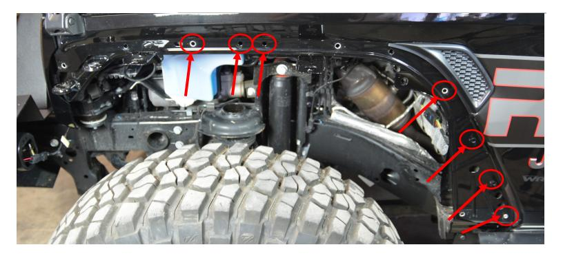
With all the nutserts installed on the driver side front panel of the vehicle, start with bracket **D1** and mount it at the front of the vehicle as shown using **two** flanged 1/4" - 20 bolts through the front brackets. Install loosely.
