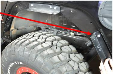
Install rear fenders onto the brackets by sliding them towards the jeep and up.
