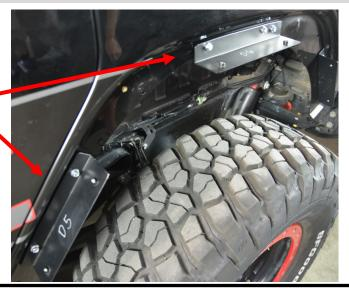
D7 will be installed at the rear of the fender well on the lower portion using **two** 1/4" - 20 flanged bolts.
