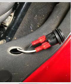
Push the button back into the hole and it should pop into place.
