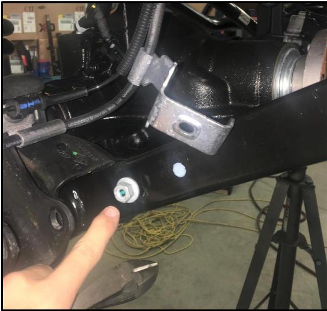
Remove Brake Lines from Arms
