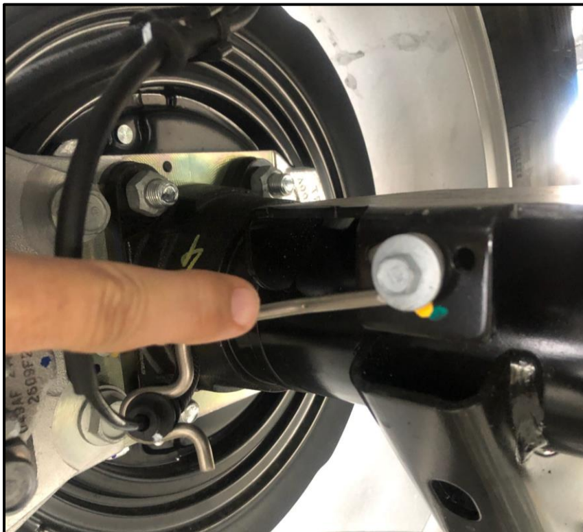
Brake Line Wire Form to be Removed
