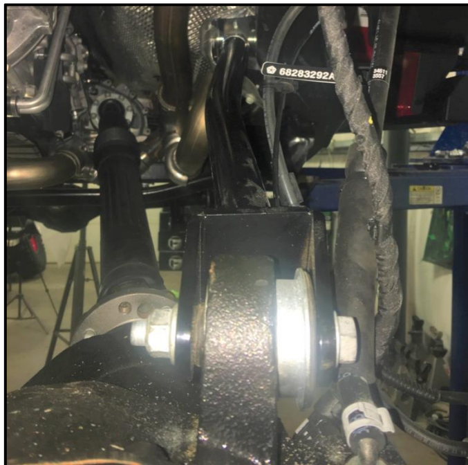
Driver Side Front Upper Arm Showing Proper Bend Orientation (Away from the frame)
