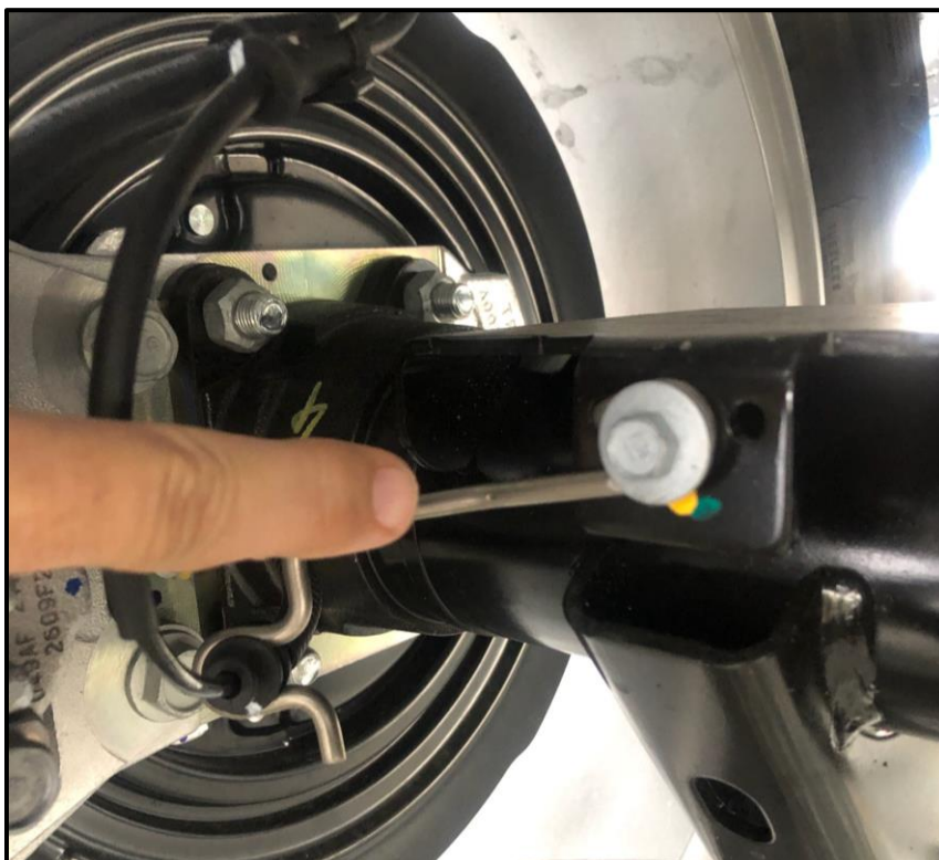
Brake Line Wire Form to be Removed
