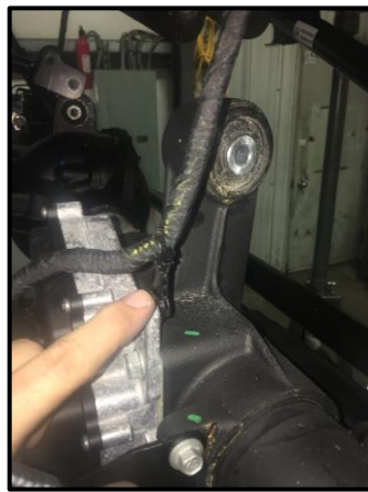
Remove Brake Lines from Arms
