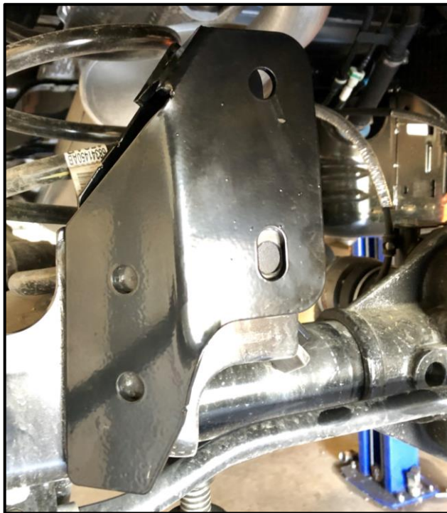
Driver Side Holes to Be Drilled
