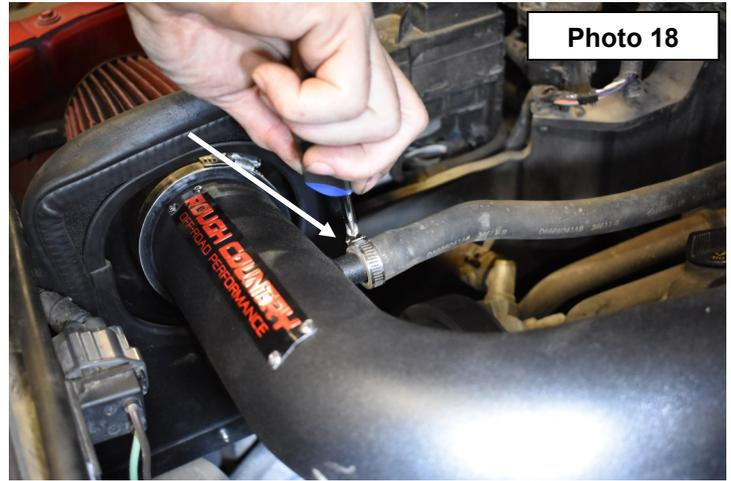
17. Install the air filter as shown with supplied hose clamp and tighten using a flat head screwdriver. **See Photo 19.**
