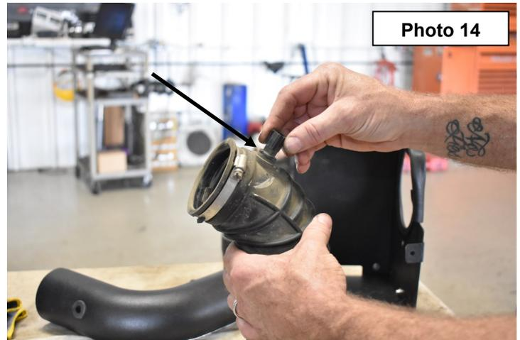
13. Install the supplied grommet in the new intake tube and install the air temperature sensor in the tube as shown in **Photo 15**. Sensor will simply push into the new grommet.
