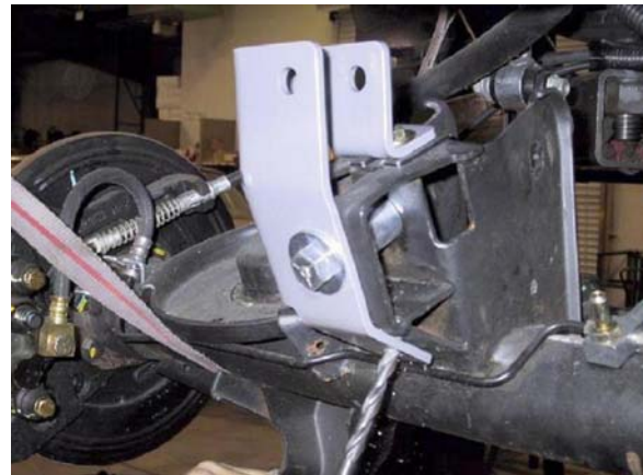
Photo 1 (TJ set up for stock track bar)
