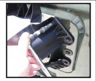
Step 3. Install the CB Antenna Mount using the supplied hex bolts, lock washers, flat washers. Torque bolts to 10 ft-lbs. Remount the spare tire after CB Antenna installation is complete.
