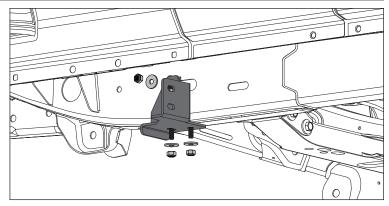
3. Remove two M10 nuts from body mount in front of rear wheel. Loosely install Rocker Guard on studs using factory M10 nuts.
