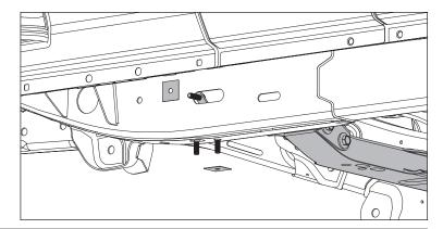
2. Install Mounting Bracket on vehicle frame using supplied M10 washers and lock nuts.
