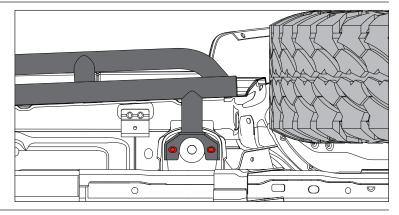
4. Attach Rocker Guard to Mounting Bracket using supplied M10 hardware. Once attached, tighten all mounting hardware.
