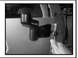
2. Locate the driver side door strap that limits the door opening. Remove the strap from the hook located inside the vehicle. **NOTICE!** The door can swing open into the vehicle once the strap is released potentially causing damage to your vehicle.
