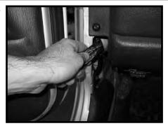
3. Remove the nuts from the bottom of each factory hinge pin. Set these nuts aside to be re-installed on the Tube Doors. To remove the factory doors, carefully lift the door upward until the hinge pins completely clear the hinges. Store OE doors in a safe place.
