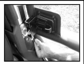
2. Drill a 3/32" hole in the Tube Door and attach the bumper with the supplied sheet metal screw. Do not overtighten. The attachment screw can be loosened or tightened as necessary to adjust the length of the Anti-Rattle Bumper.
