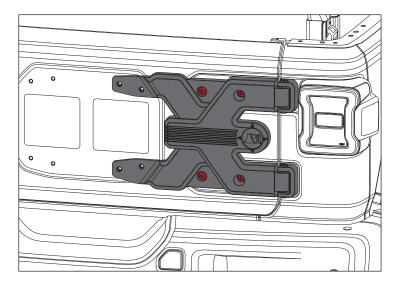
14. Install spare tire mount using factory hardware and supplied Spacer Plates on drivers side.
