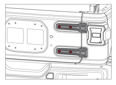
11. Without opening tailgate, remove six bolts securing factory hinges to body and remove hinges.
