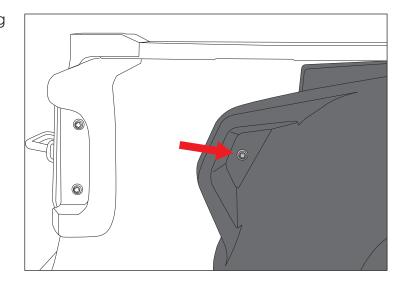
6. Starting toward front of vehicle, lightly pry trim panel out of place. Trim panel snap locations may vary between different models.
