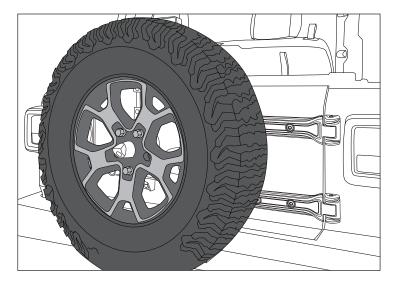
9. Using 13mm socket, remove eight factory bolts securing spare tire mount and set it out of the way.
