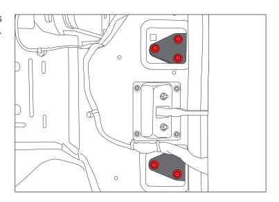
12. Insert Spartacus Hinge Casting in body openings and loosely install using six factory bolts removed in step 11.
