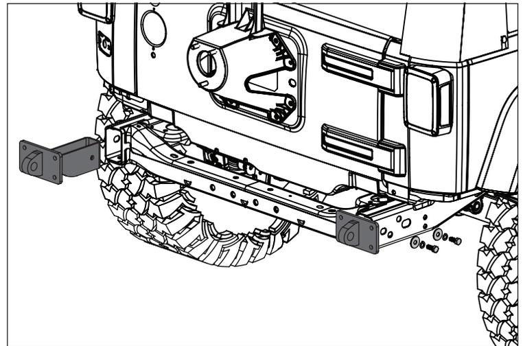
3. Install Spartan Rear Bumper on Mounting Brackets using remaining M12 hardware. Align bumper with body and fully tighten Mounting Bracket hardware.
