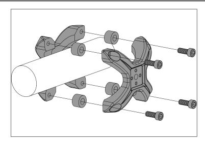
2.Slide Grip onto Grip Shaft. Using supplied M8 Bolt, loosely attach Grip Shaft and Base to X-Clamp.
