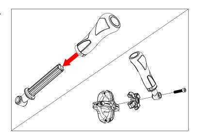
3. Adjust X-Clamp and Grip according to personal preferance. Tighten M8-35mm Socket Head bolt to 12ft-lbs. Tighten M6 X-Clamp hardware to 4ft-lbs.
