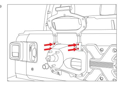
3. Remove seven screws securing backing plate to third brake light mount.
