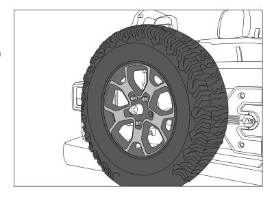
2. Remove four screws securing factory third brake light mount to tire carrier.
