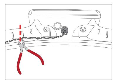
5. Install LED Third Brake Light Ring on tire carrier.
