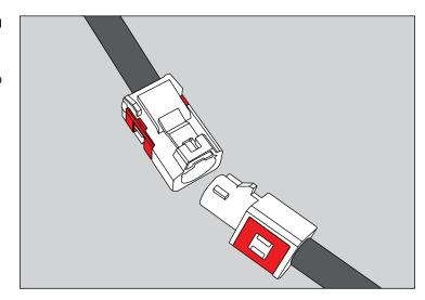
12. Connect CB Radio Cable to CB radio. Use supplied Double Female CB Adapter if necessary to connect to another CB cable.
