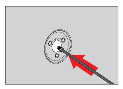
5. Install Antenna Stud on Antenna Mount. Insert Antenna Cable through Antenna Mount and Gasket and connect to Antenna Stud.
