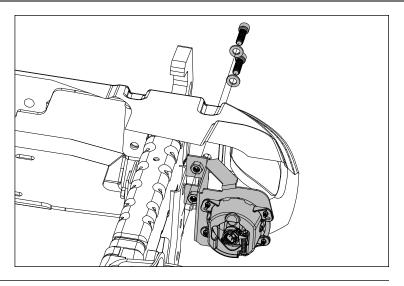
10. Position Tube Overrider and Rubber Spacer to align with Overrider Mounting Bracket and Bumper Shell. Using supplied M10 Nut and Washer, loosely attach Overrider.
