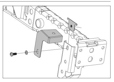
8. Position Bumper Shell and Tow Hooks into place on vehicle's frame rails. Using supplied M12 hardware and Nut Plates, loosely attach Bumper Shell and Tow Hooks using center four holes.
