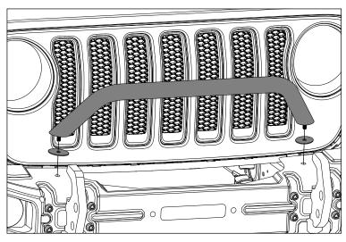
11. Attach fairlead to Bumper Shell and finish completing Winch installation.
