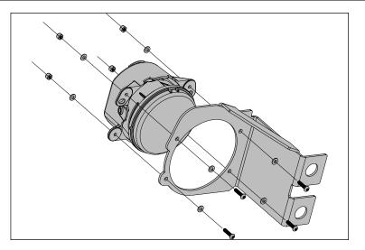
3. Using supplied M10 hardware, loosely attach Winch Tray Bracket to Winch Tray.
