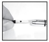
Step 3. Align the hole in the dipstick, sleeve and handle. Insert the pin removed from the factory handle using a small punch to set the pin.
