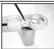
Step 2. Install the small sleeve over the end of the dipstick. Insert the dipstick and sleeve into the handle. Align the hole in the dipstick, sleeve and handle.
