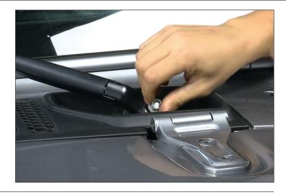
2. Remove cowl grille, pry on one corner to release a clip. Then continue to pull up and release the remaining clips.
