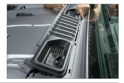
5. Attach the light bar mount. Depending on the size of the light bar you are mounting the mounts could point in or out. Place mount in front of the Hood hinge mount and tighten using the black Teflon coated M8 hardware provided.
