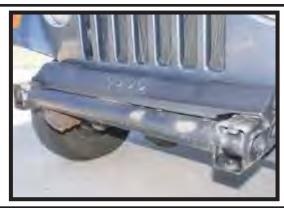
Step (2) Position the new front bumper up to the frame and line up the holes to factory mounting locations. Using the stock bolts and supplied flat washers secure bumper to vehicle.
