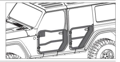
4. Close Tube Door and tighten Hinge Pin hardware. Install Check Strap and cycle Tube Door open and closed to ensure Hinge Pins are properly aligned and fully seated in door hinge.
