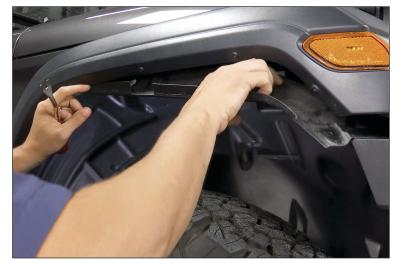
2. Remove the lower fender panel located at the rear bottom of the fender. It's held in with two plastic trees.
