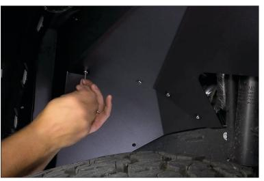
15. Now to finish install attach the remaining finish panels. The Lower Splash shield attaches to the bottom of the Firewall Panel. It requires two U-clips attached to the shield and the shield placed behind the Firewall panel and then attached with Allen Head Bolt and washer.
