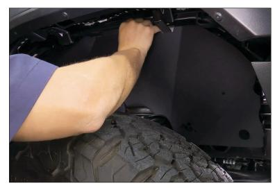
9. Now begin attaching allen head bolts with flat washers to the spring clips on the Firewall panel. Don't fully tighten at this point.
