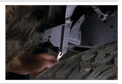
3. For Passenger side only insert the bolt plate through the fender frame located towards the top rear of the fender. The Drivers side will use a standard bolt for this mounting location.
