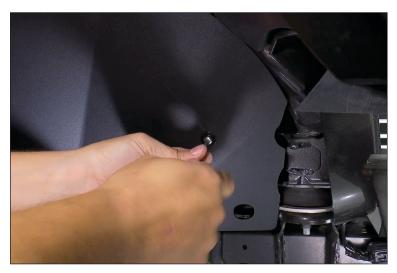
12. Now for the last mounting point attach the upper mounting tab of the main panel to the fender bracket of the Jeep using a allen head bolt with washers and nut. Adjust the panel now that all the hardware is in place. Assure the panels are not rubbing the frame or other components and now fully tighten hardware starting here with the upper mounting tab.
