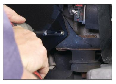
8. Now attached the rear self tapping screw to the Jeep body. That completes install.
