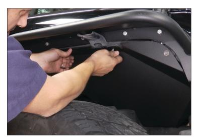
6. Now tighten these three bolts starting with the two upper bolts. Start here so it draws the panel up into position. DO NOT use power or air tools to avoid striping hardware or damaging panel.
