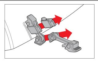
2. Remove the pivot base from the Aluminum Hood Catch assembly.
