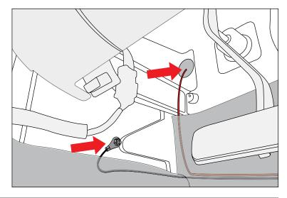
2. Place one 9" LED Tube under dashboard on each side. Attach two Mounting Tabs to each LED Tube and remove red tape backing. Press and hold each Mounting Tab to metal bar underneath dashboard for 30 seconds.
