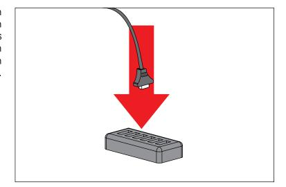
6. Run all wires under carpet and tuck underneath edge of center console. Hide Connector Block behind dashboard as shown on right. If desired, attach Hook and Loop tape to back of Remote and front of lower console panel.
