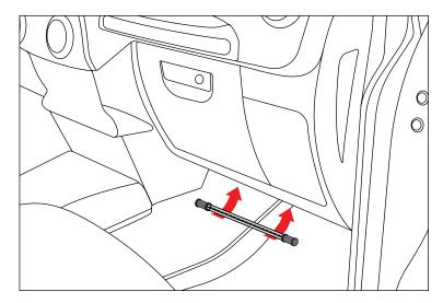
3. Place one 9" LED Tube under each front seat. Attach two Mounting Tabs to each LED Tube and remove red tape backing. Press and hold each Mounting Tab to bottom of seat for 30 seconds.
