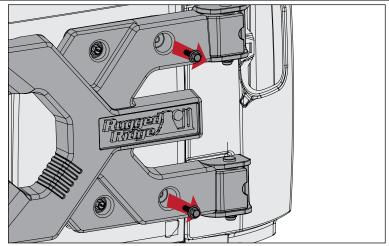
2. Align top top mounting points on Jack Mount Bracket with mounting holes in Tire Carrier. Secure with provided M10 hardware and spacers.
