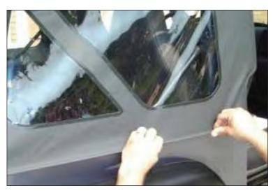
17. Install tailgate bar in receiver on each side of tailgate opening and insert rear window into "C" channel of tailgate bar.
