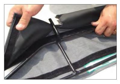
21. Use tab sewn into door skin to work top rear corner of frame into door skin between hook and loop flap. Ensure top of door skin is straight and fasten hook and loop strips tightly around frame. Once door skin is installed on frame, tab may be removed from skin using scissors.
