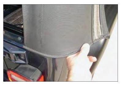
11. Wrap and fasten hook and loop strips around center bow.
