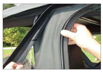
14. Locate plastic strips on each side of top and insert into door surrounds above door opening.
