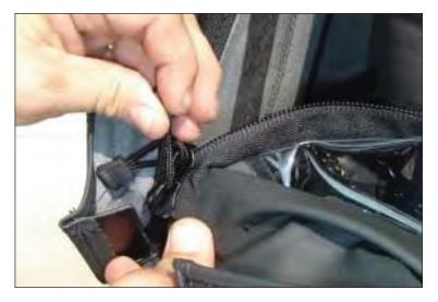
19. Remove fabric upper doors from vehicle. Using razor blade, cut stitching on old door covers and remove from frame.
