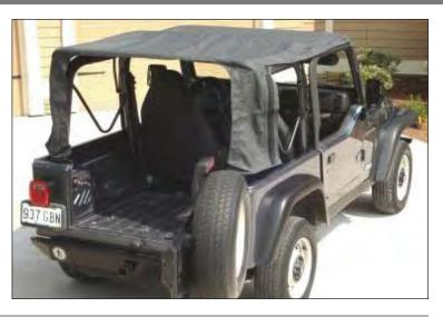
10. Ensure center bow is centered in hook and loop flap but DO NOT fasten at this time. Pull down and insert rear corners of soft top into belt rail. Secure header to windshield frame at this point.
