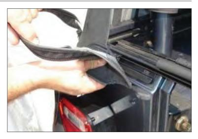
18. Start zipper of rear window. Hold up window and finish zipping rear window to top. Ensure tailgate bar is centered and securely fastened. Tuck flaps on rear window under soft top fabric.
