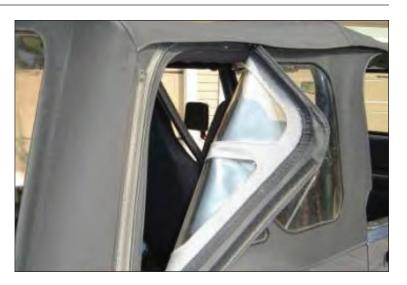
2. Release windshield latches on front header. DO NOT lower top at this point. Pull down and out on corners to release top from belt rail. Repeat for opposite side.
