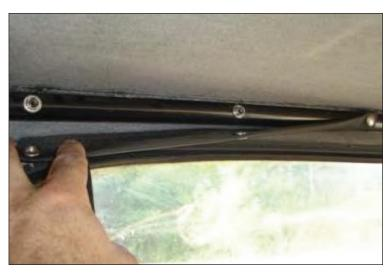
5. Lower soft top onto tailgate. Remove screws that fasten soft top fabric to corners of windshield header and set aside for later use.
