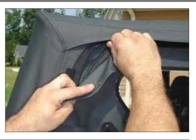
16. Start at rear of vehicle and roll plastic lip along belt rail. Fasten hook and loop strips that connect rear of side window to soft top.
