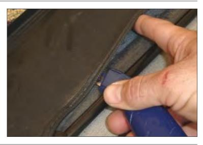
20. Unzip windows and separate hook and loop fasteners on new door skins. Lay door skin on flat surface with outside facing down. Start by working lower rear corner of door frame into pocket in lower rear corner of door skin. Proceed to lower and top front. Ensure top front corner of frame is between hook and loop flap of door skin.
